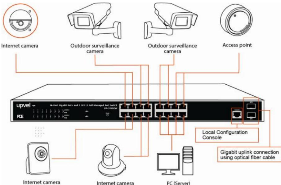
After connecting all the devices required, you can configure various features of the switch using its Web management interface. Management features include conditional monitoring of the PoE power supply (available power of ports, power supply delay, priority, and scheduling), Port Mirroring, broadcast storm protection, VLAN (tag/port), QoS, TCP/UDP packet filtering, Spanning Tree, Port Trunking, DHCP Relay, IGMP Snooping, SNMP, and many more.
